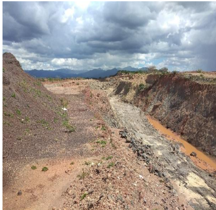
Figure 4-4: Overburden material from blasting operation piled near the open pit
