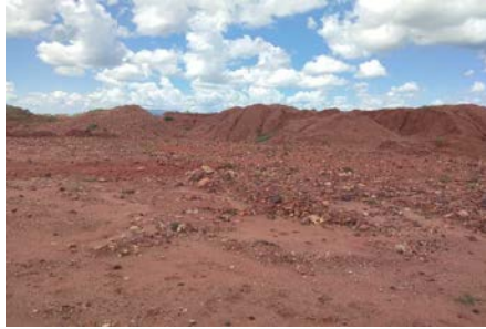
Figure 4-5: Overburden material as a result of the extraction of alluvial iron ore
