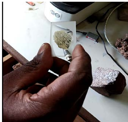
Figure 3-13: Polished sample ready for analysis
