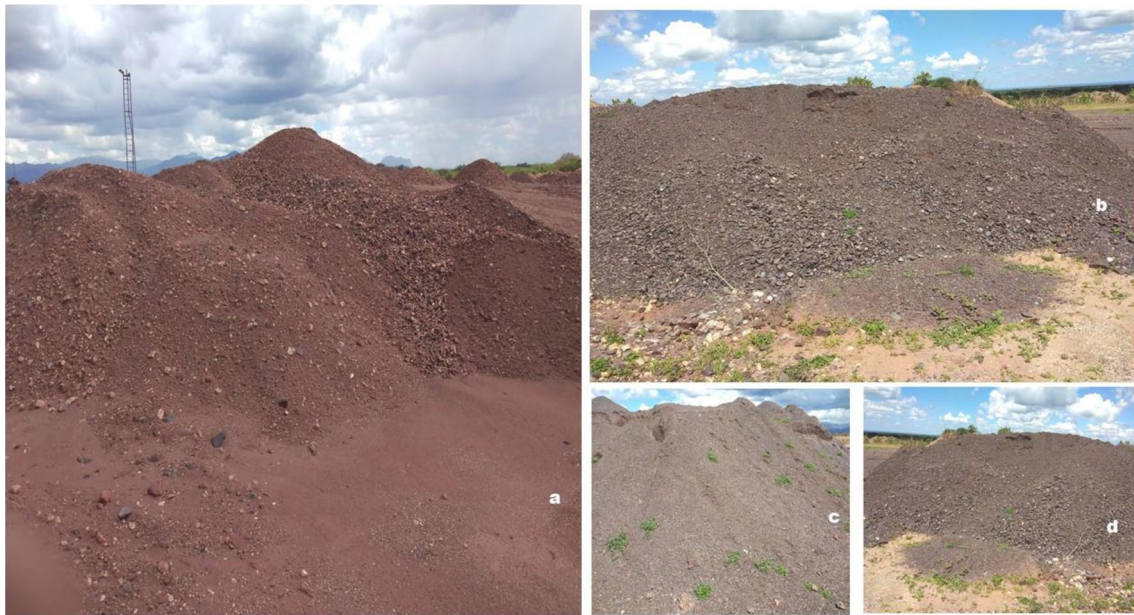
Fig. 14 Mine wastes at Samrudha resources Mine; a Overburden material, b Waste dump, c Stockpiled iron ore fines and, d Waste rock dump
