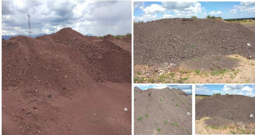
Figure 4-10: Mine wastes at samruddha resources kenya limited iron ore mine; a. Overburden material, b. Waste dump, c. Stockpiled iron ore fines, and d. Waste rock dump. Waste rock is generally excavated and mined rocks during access from ore and includes rocks resulting from blasting operations (Kakaie et al., 2019). These waste rocks are usually dumped in non-designated waste dumps around the SRKL Iron Ore Mine mining area. The overburden material at SRKL Iron Ore Mine is mainly topsoil, and rocks dozed off during the opening up of new open pits, as shown in Figure 4-11. The overburden material is piled on the sides of the mine and constitutes solid mine waste produced during mining operations under consideration in this research.
