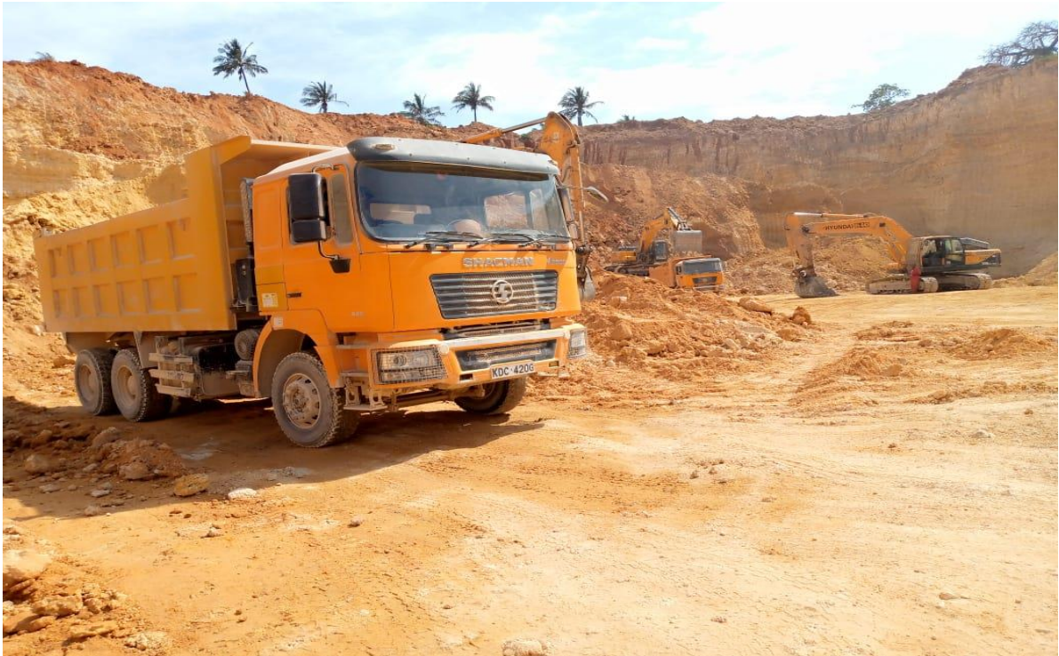
Figure 4.2: 3 m 3 Bucket Capacity Shovels Loading into 25 tonnes Capacity Trucks at the Quarry
