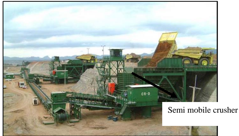
Figure 1.4: Semi-Mobile IPCC system
